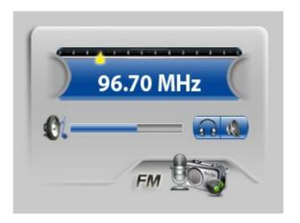
Press the [CH+]/[CH-] buttons to manually search FM programs. Pressing [CH+]/[CH-] for about one second will start the auto channel search feature.
